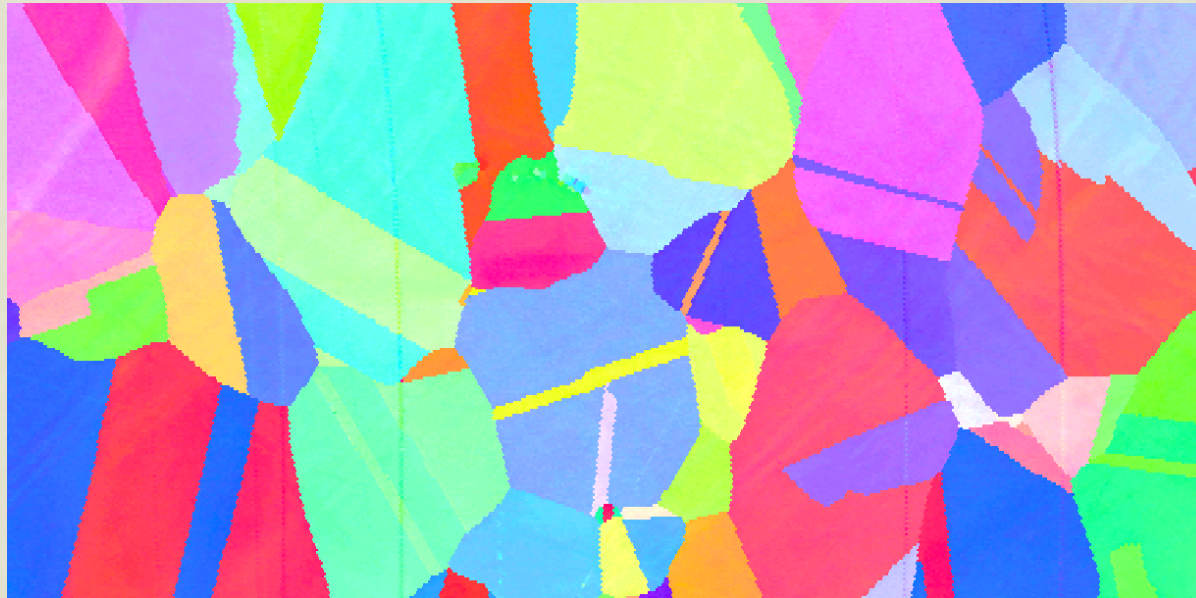
Orientation map of an Copper sample
